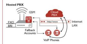
If the connection to the cloud PBX breaks, the SBA-App jumps in as local replacement PBX.
