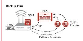
In case of a failure of the central PBX the SBA-App takes over rudimentary telephony features.
