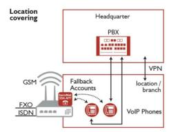
If the connection to the cloud PBX breaks, the SBA-App jumps in as local replacement PBX.
